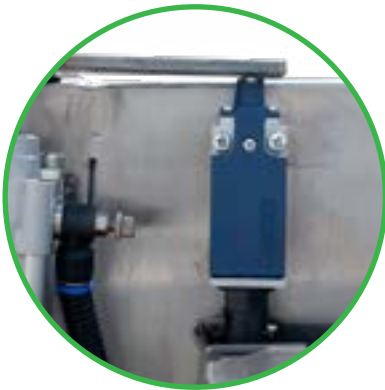
DOOR OPENING SENSOR
